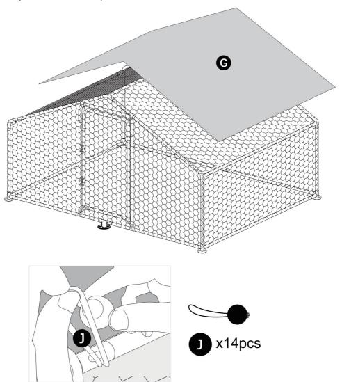
Use a bungee cord to pass through the hole in the rainproof cloth to secure the rainproof cloth.
