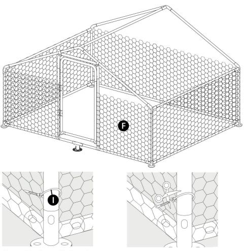
Use cable ties to fix the wire mesh to the iron pipe.
