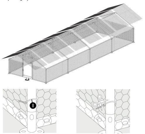
Use cable ties to fix the wire mesh to the iron pipe.
