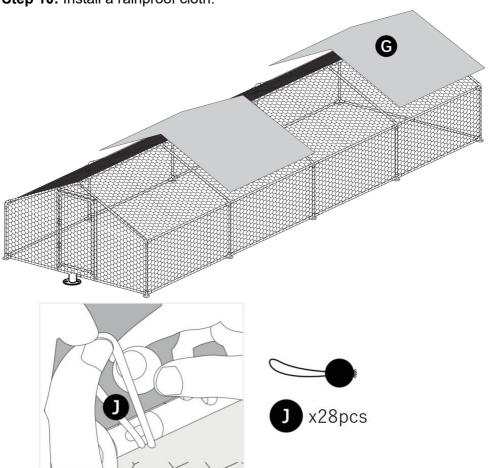
Use a bungee cord to pass through the hole in the rainproof cloth to secure the rainproof cloth.
