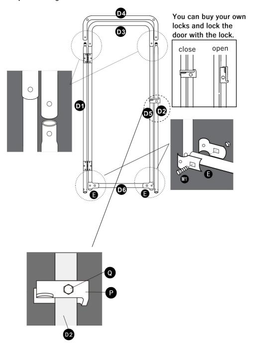
Step 6: Contact the door with the frame.
