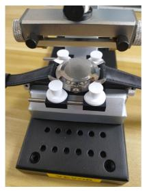
Installation of the 5700 watch machine ③: fixation of the case ②: You need to remove all the watchband before using the second way. Each of the white case fixed seats of the same size are directly inserted into the console of the 5700 watch machine. After putting the case into the case, tighten the screws at both ends to make the case fixed.
