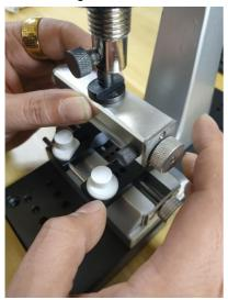
Installation of 5700 opener 3: fixed 1 of the case: Install the black base on the operating table of 5700 opener, and insert the four fixed heads into the black base in turn.
