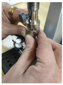
5700 open meter machine used to open the Rolex / table table back cover ③: after the 5700 open meter machine steering wheel press, make the 5538 open meter mold and the Rolex / table back cover teeth grain close contact, and then rotate the steering wheel counterclockwise, the back cover rotation open.
