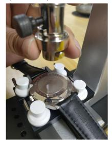
②: Connect a 5538 meter opener mold corresponding to the rear cover size (6 in total) with the connector head.
