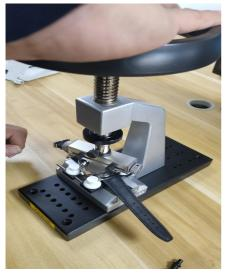
5700 open machine used to open the Rolex / Di tuo table back cover method 1: speak 5538 open device in the connector is installed on the 5700 open machine.
