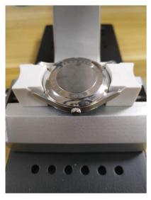
5700 open machine installation ④: after the steering wheel is pressed, make the ends of the black steel teeth embedded in case back cover relative two grooves (generally common spin bottom type back cover will have six grooves), steel teeth card into the groove, tighten the screws at both ends of the connector, make the steel teeth tightly stuck the case on the back cover groove, rotating 5700 open machine steering wheel, can make the case back cover rotation open.
