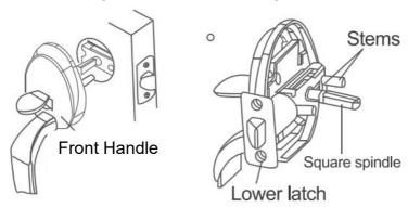
Place the front handle with stems and square spindle into the latch as shown. Press tightly against the door face.
