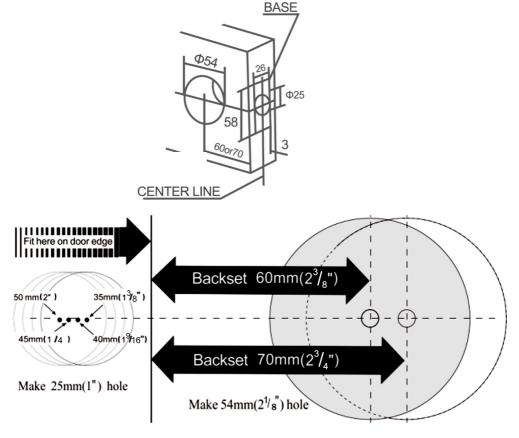
A: Fold the template over the edge of the door and mark the site 60mm or 70 mm of holes.
