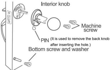
After the front handle is in position, install the interior knob and tighten screws. Insert screw through washer and into bottom hole tighten firmly.
