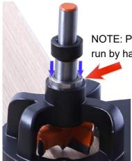
NOTE: Press down slowly and test run by hand after installation.
