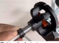
Tighten the fastening screws.
