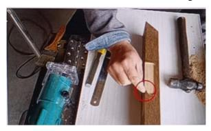
7. Use a chisel to chisel off the curved and reserved sections, makina sure the edges are flat.
