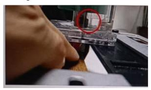
5. Slotting with the wooden router.
