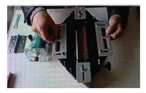
3. Adjust the screws on the four sides to determine the working range of the wood router.
