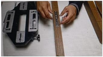
2. Put the slotted retainer on the wooden door and fix it (Clamp by tightening the black nuts.)
