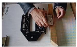
2. Put the slotted retainer on the wooden door and fix it (Clamp by tightening the black nuts.)
