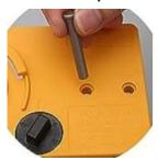
6. Use the clamp to fasten the jig and install the cutter.
