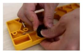
**NOTE:** For drilling 26mm hinge holes, install 26mm auxiliary accessories on the stop block on the back of the main body.
