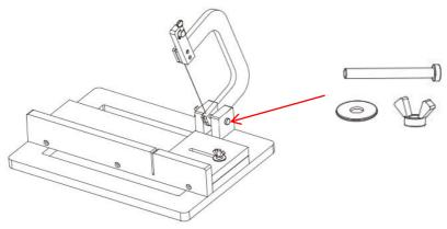
4. After loosening the butterfly nut, the cutting length limit block can be adjusted to select the cutting length you need.
