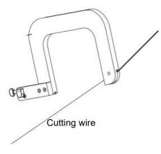
③Pass the new steel wire through the small round gasket and tighten the bolt here with the screwdriver.
