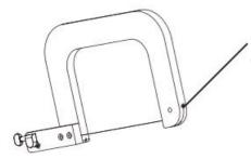
Loosen the bolt here with a screwdriver.
