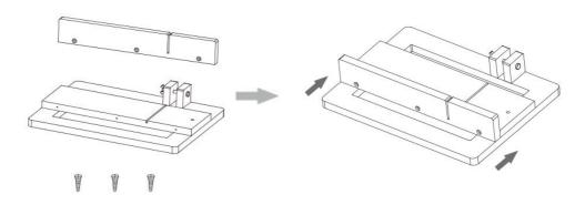
2. The bolt is threaded from the bottom of the base, and then the cut length limit block, gasket and the butterfly nut are put down in turn for assembly.
