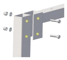
Place upper crossbar (3) at the top of the vertical bar (1). Insert retaining screws T4 (2 for each side). Tighten screws with nut cap using wrench keys. Repeat for the other side.
