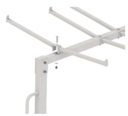
Place first chair hook on crossbar (3). Align hooks hole with crossbar (3) hole. Insert crossbar retaining screw T4 (1 for each). Tighten screw with nut cap using metal key. Repeat for all the other 5 hooks.
