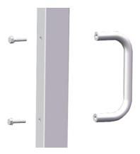
Finally,attach your side handle.Place handle on vertical bar. Insert retaining screws T2 (2 for each handle). Tighten screws using the hex key.Repeat for the second handle.
