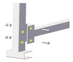
Place a lower crossbar (4) at the end of the vertical bar (1). Insert retaining screws T4 (2 for each side). Tighten screws with nut cap using wrench keys. Repeat for the other side.
