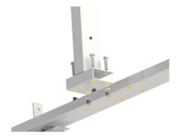
Take vertical bar (1) and place it in the middle of the bar(2). Make sure the rail part of the bar faces in. Insert retaining screws T3 (4 for each bar). Tighten screws with nut cap using wrench keys. Repeat for the other side.
