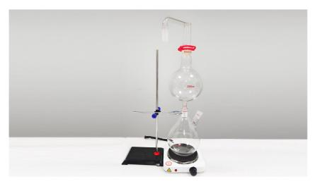
5. Install the coil condenser and fix it with a claw clamp;
