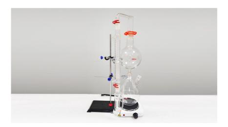
7. Install the thermometer adapter and the thermometer at the branch of the two-necked flat bottom flask.
