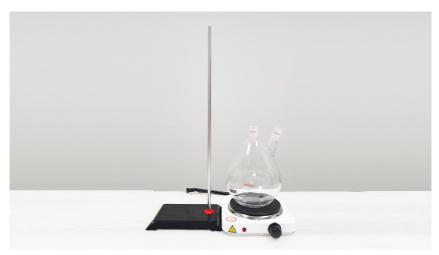
2. Fix the flask with a flask clamp;
