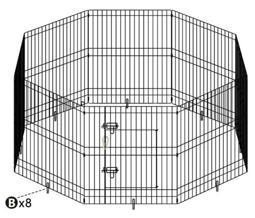
**NOTE:** When the fence needs to be fixed outdoors, the ground nail (part B) can be inserted into the ground as shown in the figure.
