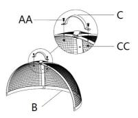
**Step 6:** Assemble the part and handle C assembled in Step 4, using 2 AA screws and 2 CC nuts.
