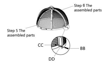
**Step 7:** Assemble the parts of Steps 5 and 6 with 2 BB screws, 2 CC nuts and 2DD annular tubes.
