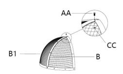
**Step3**: Assemble B and B1 mesh with **Step4**: Assemble B and B2 mesh 4 AA screws and 4 CC nuts
