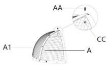
**Step 1**: Assemble A and A1 mesh with **Step2**: Assemble A and A2 mesh with 4 AA screws and 4 CC nuts
