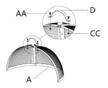
**Step 5:** Assemble the part and handle D assembled in Step 2, using 2 AA screws and 2 CC nuts.
