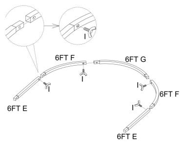
Step 2: Assemble Part B as shown using hardware I.
