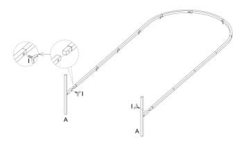
Step 4: Assemble Part "6FT C" & "6FT D" as shown using hardware I. Then use part J to install them onto the frame you completed in the previous step. The position of the assembled part I on the component before locking part J can be adjusted according to your needs.
