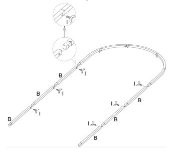
Step 3: Assemble Part A as shown using hardware I.
