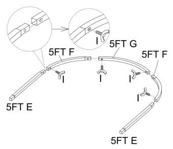
Step 2: Assemble Part B as shown using hardware I.
