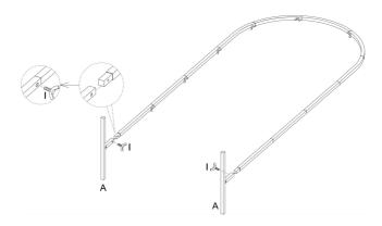
Step 4: Assemble Part "6FT C" & "6FT D" as shown using hardware I. Then use part J to install them onto the frame you completed in the previous step. The position of the assembled part I on the component before locking part J can be adjusted according to your needs.
