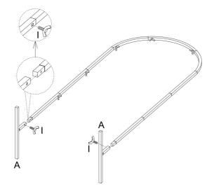
Step 4: Assemble Part "5FT C" & "5FT D" as shown using hardware I. Then use part J to install them onto the frame you completed in the previous step. The position of the assembled part I on the component before locking part J can be adjusted according to your needs.
