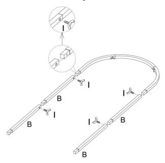
Step 3: Assemble Part A as shown using hardware I.
