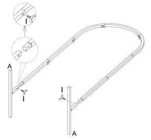
Step 4: Assemble Part "4FT C" & "4FT D" as shown using hardware I. Then use part J to install them onto the frame you completed in the previous step. The position of the assembled part I on the component before locking part J can be adjusted according to your needs.
