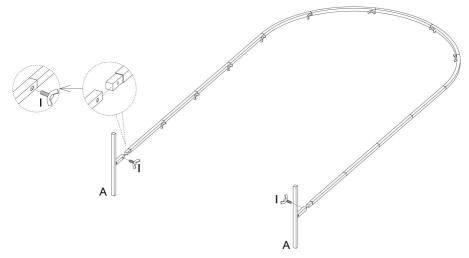
Step 4: Assemble Part "7.2FT C", "7.2FT D" & "7.2FT E" as shown using hardware I. Then use part J to install them onto the frame you completed in the previous step. The position of the assembled part I on the component before locking part J can be adjusted according to your needs.
