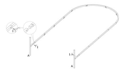
Step 4: Assemble Part "6.6FT C", "6.6FT D" & "6.6FT E" as shown using hardware I. Then use part J to install them onto the frame you completed in the previous step. The position of the assembled part I on the component before locking part J can be adjusted according to your needs.
