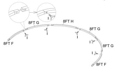
Step 2: Assemble Part B as shown using hardware I.
