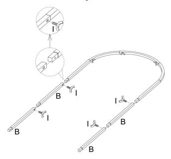
Step 3: Assemble Part A as shown using hardware I.
