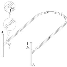
Step 4: Assemble Part "4FT C" & "4FT D" as shown using hardware I. Then use part J to install them onto the frame you completed in the previous step.
