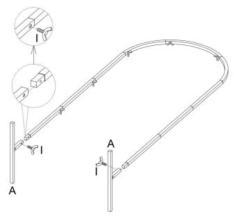
Step 4: Assemble Part "5FT C" & "5FT D" as shown using hardware I. Then use part J to install them onto the frame you completed in the previous step.
