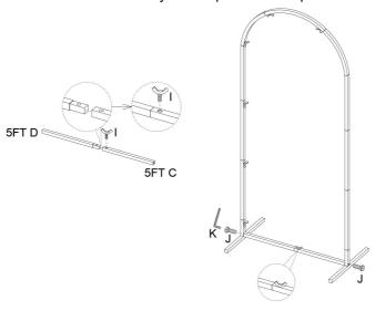
Step 5: Expand part "5FT H" and attach it to the frame completed in step 4.
