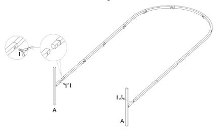
Step 4: Assemble Part "6FT C" & "6FT D" as shown using hardware I. Then use part J to install them onto the frame you completed in the previous step.
