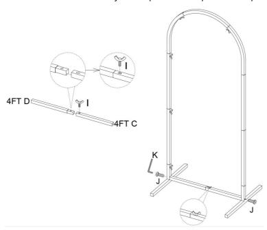
Step 5: Expand part "4FT G" and attach it to the frame completed in step 4.
