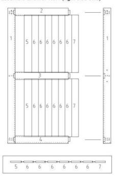
Step 3. Insert the 10 pcs of A (2-3/4" lag bolts) into No. 1 (left side stile and right side stile) and tighten them securely
