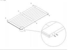
Step 5.Install the No. 8 (diagonal overlay) and No. 9 (diagonal overlay) using C (13/16" lag bolts) on the front of door, then turn the door over, install the other side.
