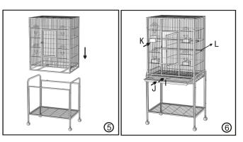
5.Put the assembled iron bird cage on the assembled iron frame, matching.
