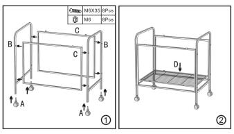
1.Take out the iron frame and assemble it with screws, and also install casters.
