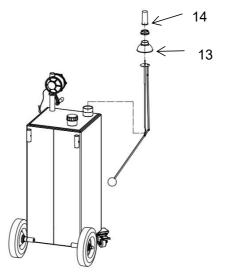
Step5: Insert the handle(2) into the tank at the appropriate position, as shown.
