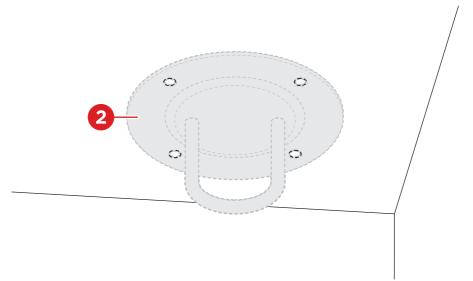
Drill four holes at the mounting location.
