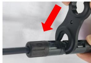
Step 1: Release the connector buckle with a tool
