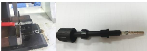
c. **Method 1:** Install the wire into the terminal slot, put it in the appropriate position of the wrench (as shown in the picture), squeeze and press the wire to complete riveting.
