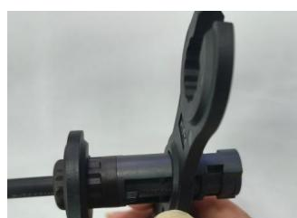
e. Place the waterproof pad in sequence, lock the teeth, and tighten the nut with tools to complete the installation.
