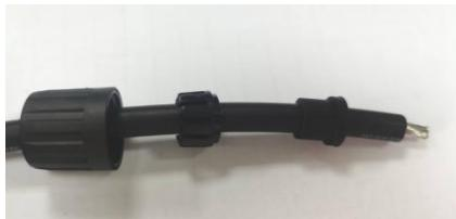
b. Put the wire in turn, tighten the cap, lock the teeth, and peel the wire after the waterproof pad. The peeling length is 10mm
