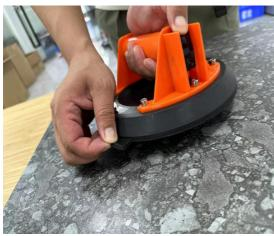
5. After the transportation process is completed, gently lift the deflation tongue or press the black deflation button to remove the suction cup.
