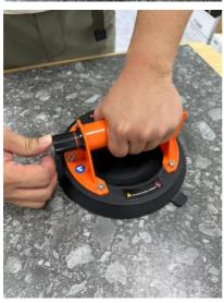
3. When operating, place the vacuum suction cup flat on the surface of the object to be adsorbed; lightly press the vacuum suction cup with your hand to ensure full contact between the rubber pad and the object's surface. Then press the inflation button until it is fully inflated and the red warning line is not visible.
