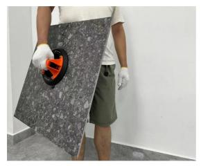
4. After complete inflation, check the red warning line to see if it has retracted. If it has not retracted, then the object can be moved.
