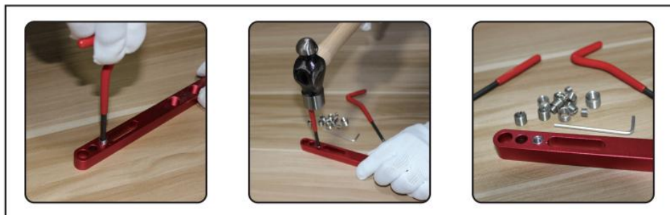
4. Screw coil into casting
