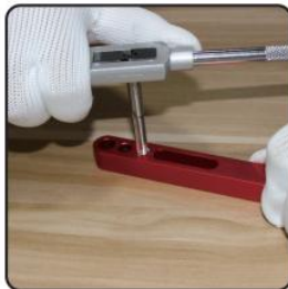
2. Tap re-drilled hole using tap supplied
