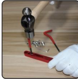
5. Using lug breaking tool, break off tag on insert
