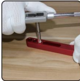
2. Tap re-drilled hole using tap supplied
