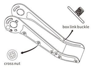
Step2:Install large side plate and small side plate on both sides and screw on cross screw nuts.
