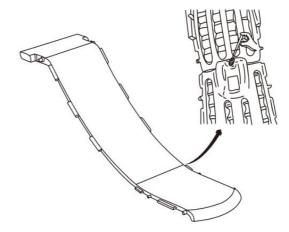
Step1:Place the slide rail (top) on the buffer plate (bottom), align the holes, and then use a screwdriver to tighten the screws from the back<sub>o</sub>
