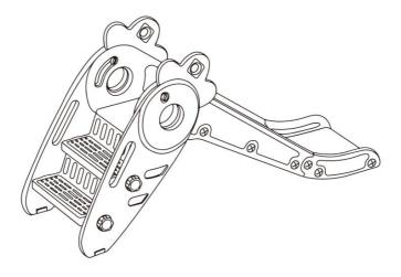
Step6:assemble the radish side plate and radish head on the other side . Screw on the fixing nut and the fixing screw .
