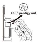
Secure the assembled staircase to the L side panel
