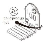
4 2 lug platform and platform baffle assembly
