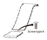
Assemble the slide EXTENSION with the Slide LARGE, and then tighten the screws.
