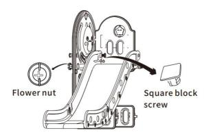
**6** Install the assembled guide rails
