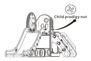
Attach the L-side plate to the other side of the slide
