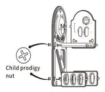
**5** Fix the assembled platform and 3-hole baffle
