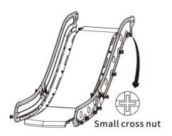
2 Secure rails on both sides of the guide rails
