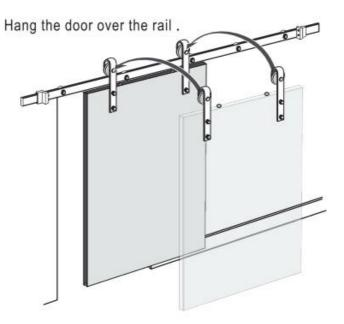
Turn the rubber ends approximately 180 degrees so that they are stuck between the door and the rail.
