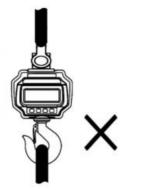
DO NOT push/pull on the loaded scale or directly on the hook!
