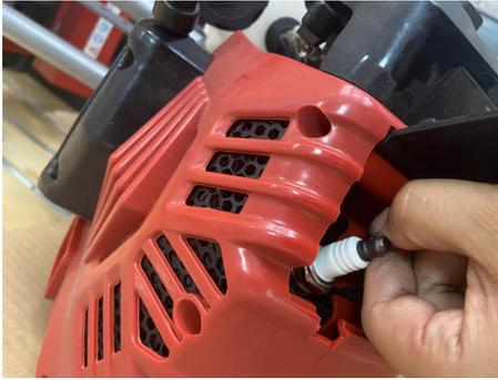
**Tighten using the wrench taking care not to over-tighten.**
