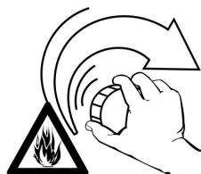
Unit vibrations can cause an improperly tightened fuel filer cap to loosen or come off and spill quantities of fuel. In order to reduce the risk of fuel spillage and fire, tighten the fuel filer cap by hand as securely as possible. See also the "Fueling" chapter in your Instruction Manual for additional information.
