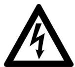
Your power tool is not insulated against electric shock. To reduce the risk of electrocution, never operate this power tool in the vicinity of any wires or cables (power, etc.) which maybe carrying electric current.
