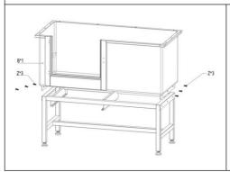
③ Use screw(Z) to fix the bottom bracket and tub(B)
