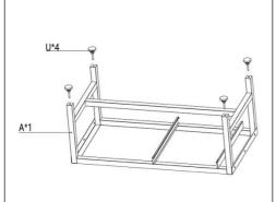
① Install the adjustable feet(U) to the bottom bracket(A)
