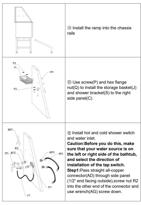
**Step2:**Align the faucet switch (H) with the connector (AD), then tighten the two nuts on the switch (H), and note that the sealing ring inside the nut is intact.
