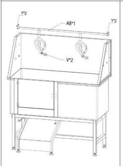
(3) Use screw(Y) to fix the crossbar (AB) to the left and right-side panel, then install the sling(V)
