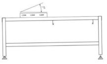
② Flip the bottom bracket, adjust the height of the feet to make sure the height of water outlet side is 1-2 degrees lower than the other side (use a spirit level to show)
