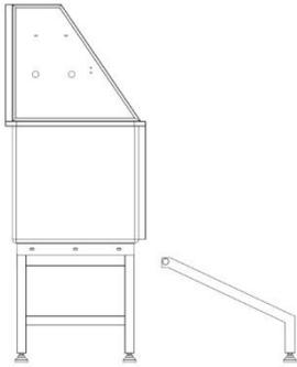
⑩ Install the ramp into the chassis rails
