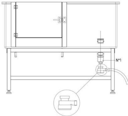
⑤ Install the strainer(N), Ensure that the sealing ring is free of dislocation and wrinkles.
