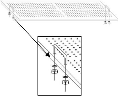
⑦ Install the handle(AF) to the water filter plate(F)
