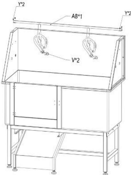
⑬ Use screw(Y) to fix the crossbar (AB) to the left and right-side panel, then install the sling(V)
