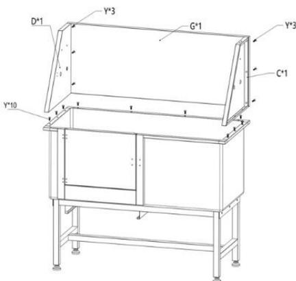
⑥ Use screw(Y) to fix the left and right side board(D&C), then use screw(Y) to fix the back panel(G), last to use screw(Y) to fix side board(D&C) and back board(G)
