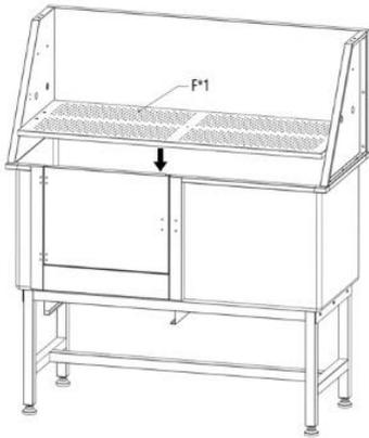
⑧ Put the water filter plate(F) to the tub(B)
