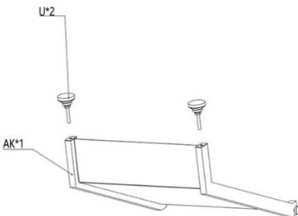
⑨ Install the adjustable feet(U) on the bottom of the ramp(AK).
