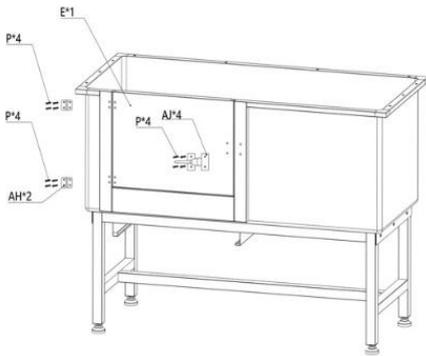
④ Use Screw(P) and hinge(AH) to fix door(E) to the tub(B), and install the latch(AJ) with screw(P)
