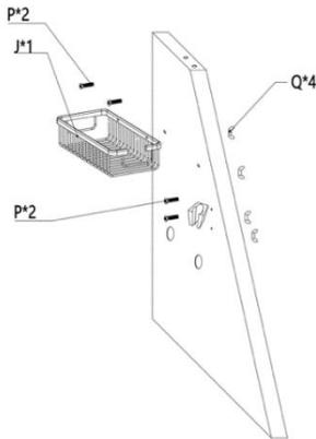
⑪ Use screw(P) and hex flange nut(Q) to install the storage basket(J) and shower bracket(S) to the right side panel(C)
