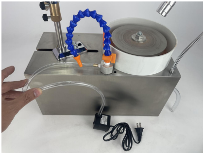
The faucet is connected to the water pump
