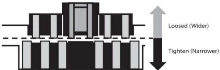
Feeding gap adjustment with one banknote
