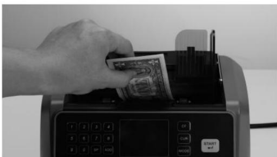
Feeding gap adjustment with one banknote
