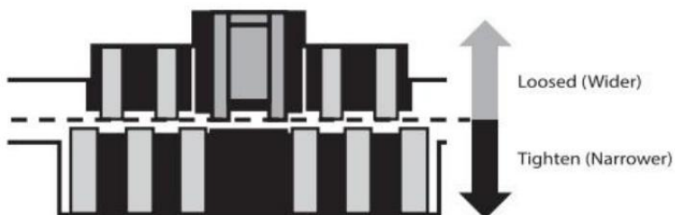
Feeding gap adjustment with one banknote
