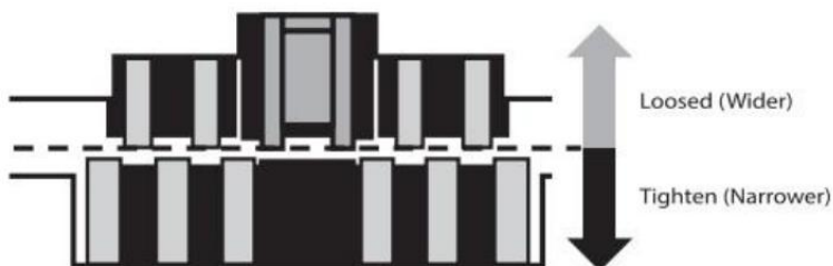
Feeding gap adjustment with one banknote
