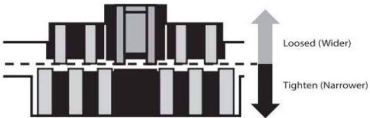
Feeding gap adjustment with one banknote
