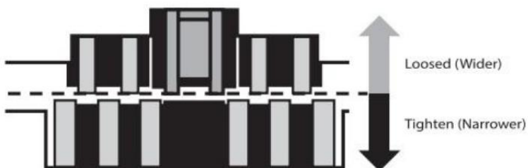
Feeding gap adjustment with one banknote
