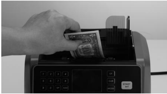
Feeding gap adjustment with one banknote
