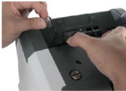
Figure 2 - 3 Banknote Guider Uninstallation
