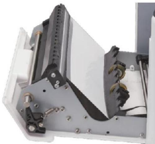
Figure 7 - 21 Place the CIS Calibration Paper
