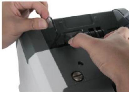
Figure 2 - 3 Banknote Guider Uninstallation
