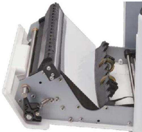
Figure 7 - 21 Place the CIS Calibration Paper
