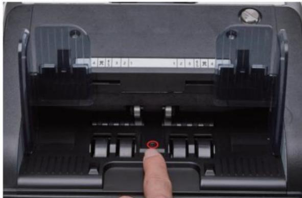
Figure 7 – 26 Touch the Hopper Sensor
