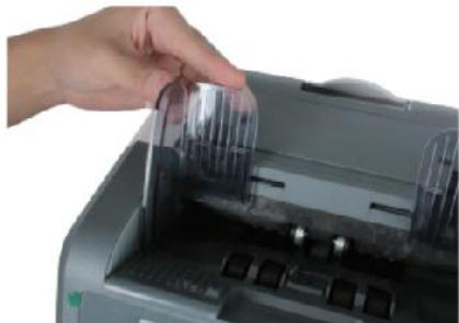
Figure 2 - 2 Banknote Guider Installation
