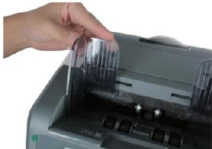
Figure 2 - 2 Banknote Guider Installation
