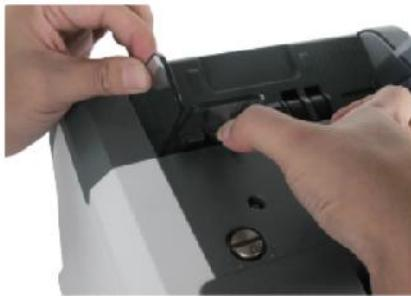
Figure 2 - 3 Banknote Guider Uninstallation
