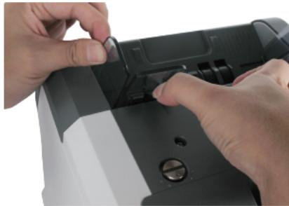
Figure 2 - 3 Banknote Guider Uninstallation
