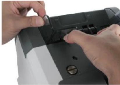
Figure 2 - 3 Banknote Guider Uninstallation
