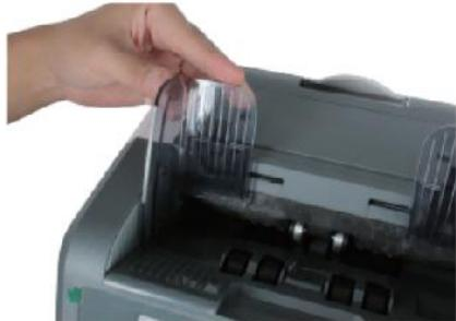
Figure 2 - 2 Banknote Guider Installation
