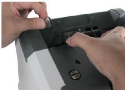
Figure 2 - 3 Banknote Guider Uninstallation
