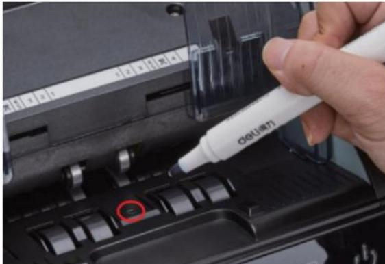
Figure 7 - 27 Use Marker Pen to Decrease the Sensitivity of Hopper Sensor
