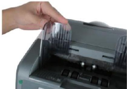
Figure 2 - 2 Banknote Guider Installation
