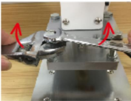
Hot stamping plate balance adjustment: First, loosen the screws in the reverse
