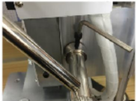
Stroke control fixed ring: Use the fixed stroke control ring to adjust the depth of
