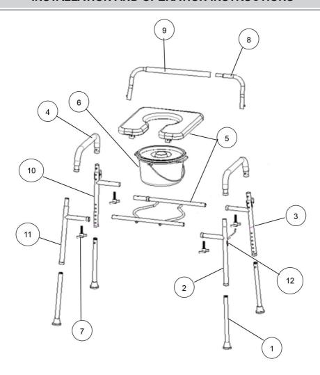
1. As shown in the figure, the four legs① are installed into the left front main frame②, the left rear main frame③, the right rear main frame⑩ and the right front main frame⑪ in turn.
