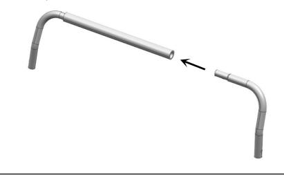
7. Insert the entire assembled backrest tube into the short tubes on either side of the rear main frame as shown.
