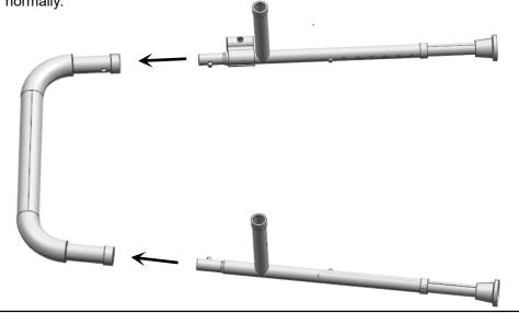
3. As shown in the figure, insert the assembled left and right main frames in line with the tube openings of the seat frame (5) (be careful not to install the seat frame and main frame in the front and rear directions in reverse).
