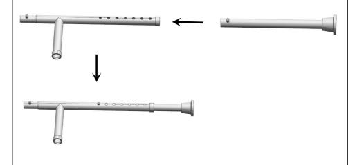
2. As shown in the figure, the assembled left front main frame 2, left rear main frame 3, right rear main frame 0, and right front main frame are put into the armrest tube 4 respectively, so that the marbles of each main frame eject normally.
