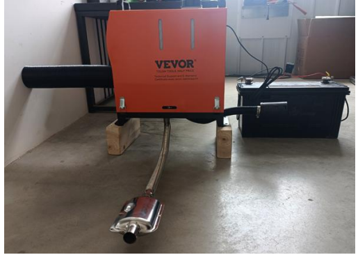
Indoor installation (wooden floor exhaust pipes need to be protected)
