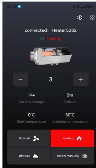
Power on status (manual mode)
