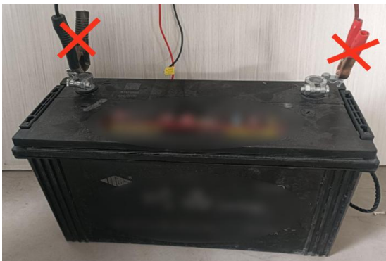
Fixing the battery clamp can easily cause poor contact
