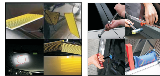
4. Place the dent lifter 3. Attach the puller tabs to the depression, wait about 2 minutes
