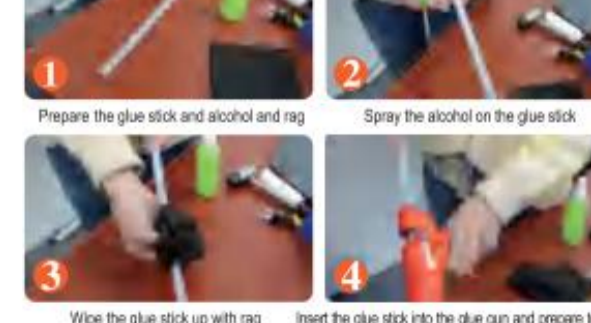
1 Prepare the glue stick and alcohol and rag 2 Spray the alcohol on the glue stick 3 Wipe the glue stick up with rag 4 Insert the glue stick into the glue gun and prepare to charge it
