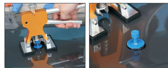
4. Place the dent lifter 3. Attach the puller tabs to the depression, wait about 2 minutes
