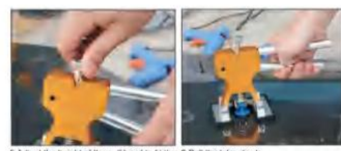
3. Adjust the height of the pull head to fit the puller tabs
