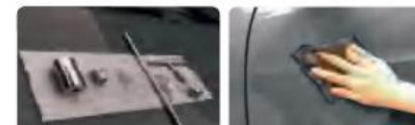
Prepare the tools You had better to clean the dent with alcohol and rag before repair.
