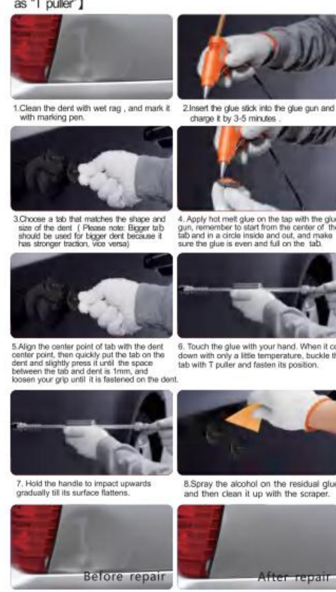
1. Clean the dent with wet rag, and mark it with marking pen. 2. Insert the glue stick into the glue gun and charge it by 3-5 minutes. 3. Choose a tab that matches the shape and size of the dent. (Please note: Bigger tab should be used for bigger dent because it has stronger traction, vice versa) 4. Apply hot melt glue on the tab with the glue gun, remember to start from the center of the tab and in a circle inside and out, and make sure the glue is even and full on the tab. 5. Align the center point of tab with the dent center point, then quickly put the tab on the dent and slightly press it. (Wait 3-5 minutes till it cools down with only a little temperature when it has strongest viscosity.) 6. Touch the glue with your hand. When it cools down with only a little temperature, buckle the tab with T puller and fasten its position. 7. Hold the handle to impact upwards gradually till its surface flattens. 8. Spray the alcohol on the residual glue, and then clean it up with the scraper. Before repair After repair
