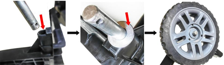
3. Insert the second steel gasket into the rod, then insert the split cotter in the hole of rod, then bend the bottom of split cotter by sharp-nose pliers.
