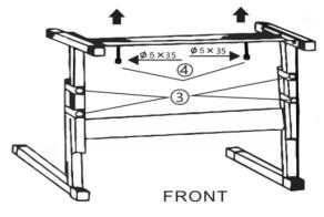
Adjust the limit screw at the same time on the left and right sides to adjust the appropriate height
