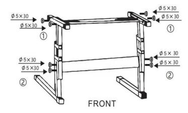
Connecting the screw hole position at the bottom of the piano body
