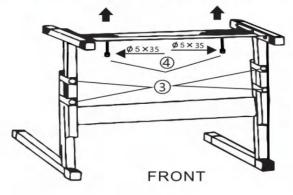
(3) Adjust the limit screw at the same time on the left and right sides to adjust the appropriate height
