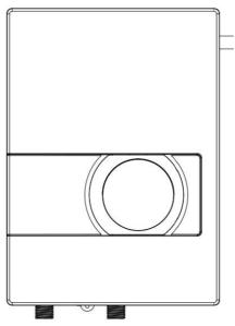
Fig 6 Tear off the installation cardboard from user manual inner page, to make 2 marks for punching; then drill 2 holes with 6mm diameter, the distance between 2 hole is 89mm. and insert 2 expansion screws in the wall and put 4\*25mm self-tapping screw into the expansion screw.
