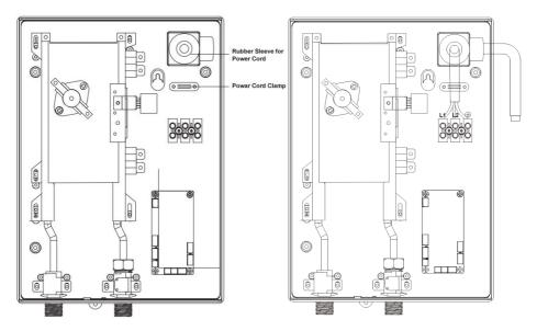
Fig 4 → Connect the cable to the terminal blocks, please notice the guidance logo below the terminal blocks. JN08 will be connected to one circuit breaker, JN13 will be connected to two circuit breakers.
