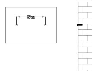
**Fig 7** Fix the appliance on the wall and put one 4\*25mm self-tapping screw into the expansion screw pass though the bottom hole to lock down the appliance.
