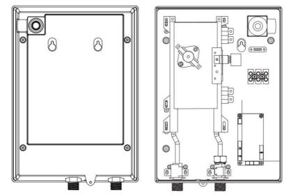
Fig 3 → Cut the top of cable protection sleeve, loosen the screw of the cable fastener.
