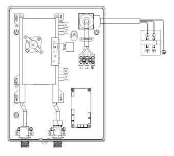
**Fig 5** Fix the front cover on appliance, fix the cable fastener and lock the 4 screws to fix the front case.
