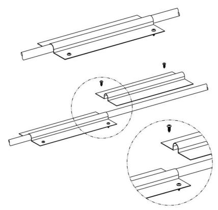
During installation, the heat transfer plate can be cut to any size at will.
