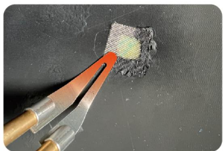
3. Use the hot smoothing head to melt stainless steel mesh into the base plastic
