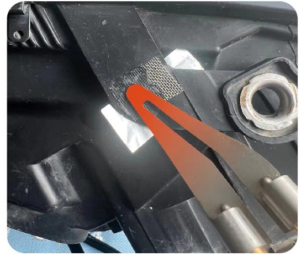
4. Use the hot smoothing head to melt into the base plastic
