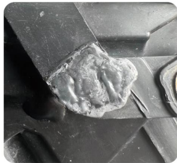
6. After completed repair, remove the metal foil
