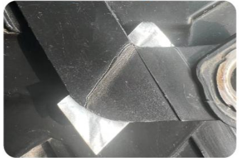
2. Stick the broken part with metal foil for easy maintenance
