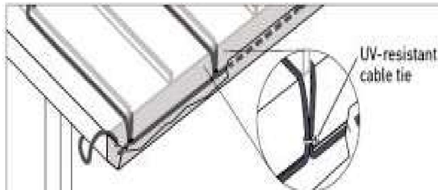
Figure 6. Standing seam metal roof
