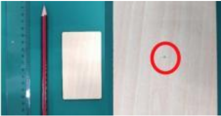
picture 1 draw a center point on the engraved object
