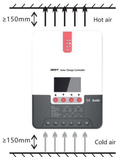
Fig. 2.1 Installation and heat dissipation
