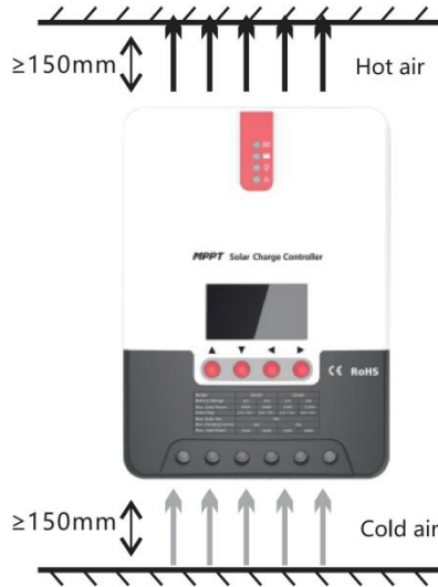
Fig. 2.1 Installation and heat dissipation
