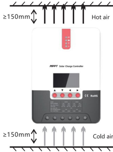
Fig. 2.1 Installation and heat dissipation
