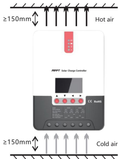
Fig. 2.1 Installation and heat dissipation
