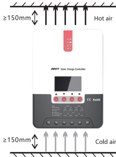
Fig. 2.1 Installation and heat dissipation
