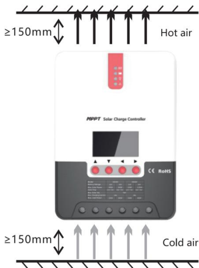
Fig. 2.1 Installation and heat dissipation
