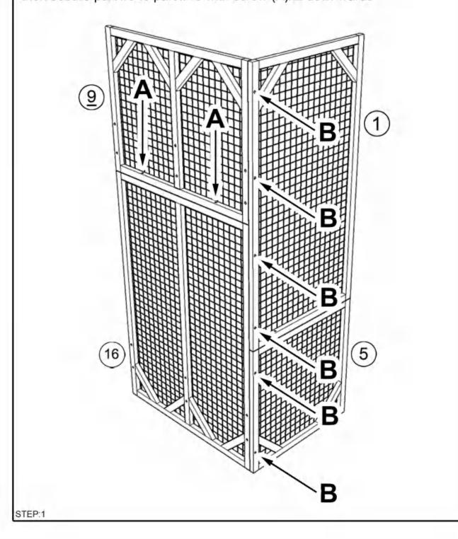
Secure part #1 to part #5 with screw (A)x2 downwards, then assemble part #4 and part #8 with screw (A) x6 as shown, please pay attention to the up and bottom orientation of part #4, the end with 2 pre-drilled holes is bottom as shown in the figure
