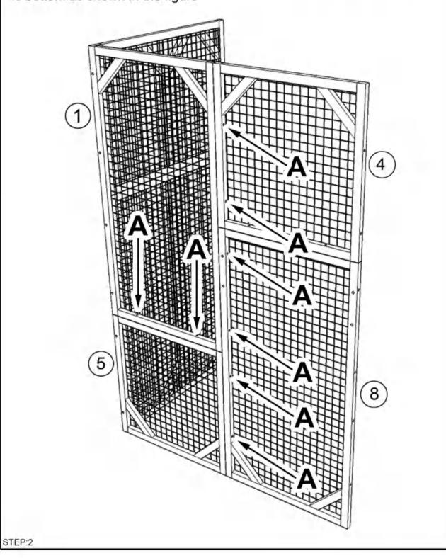
Assemble part #3 and part #7 with screw (A) x6 as shown, please pay attention to the up and bottom orientation of part #3, the end with 2 pre-drilled holes is bottom as shown in the figure, then secure part #3 to part #7 with screw (A)x2 downwards
