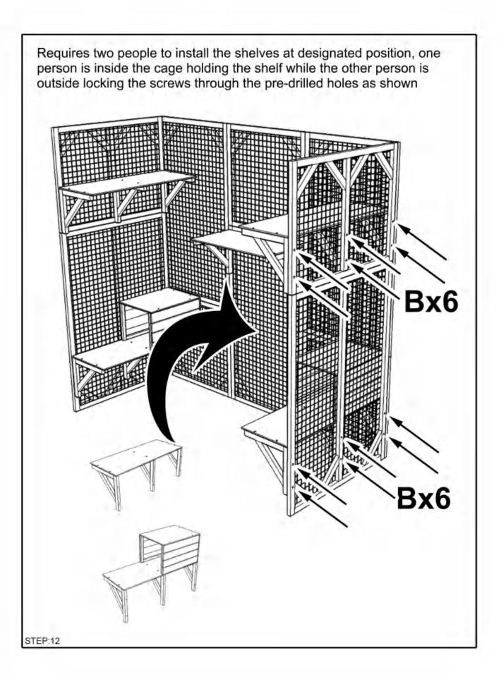
Assemble part #1 and #5, part #3 and #7 with screw (B) x12 as shown, please pay attention to the up and bottom orientation of part #1 and #3, the end with 2 pre-drilled holes is bottom as shown in the figure, then secure part #1 to part #5 with screw (A)x2 downwards
