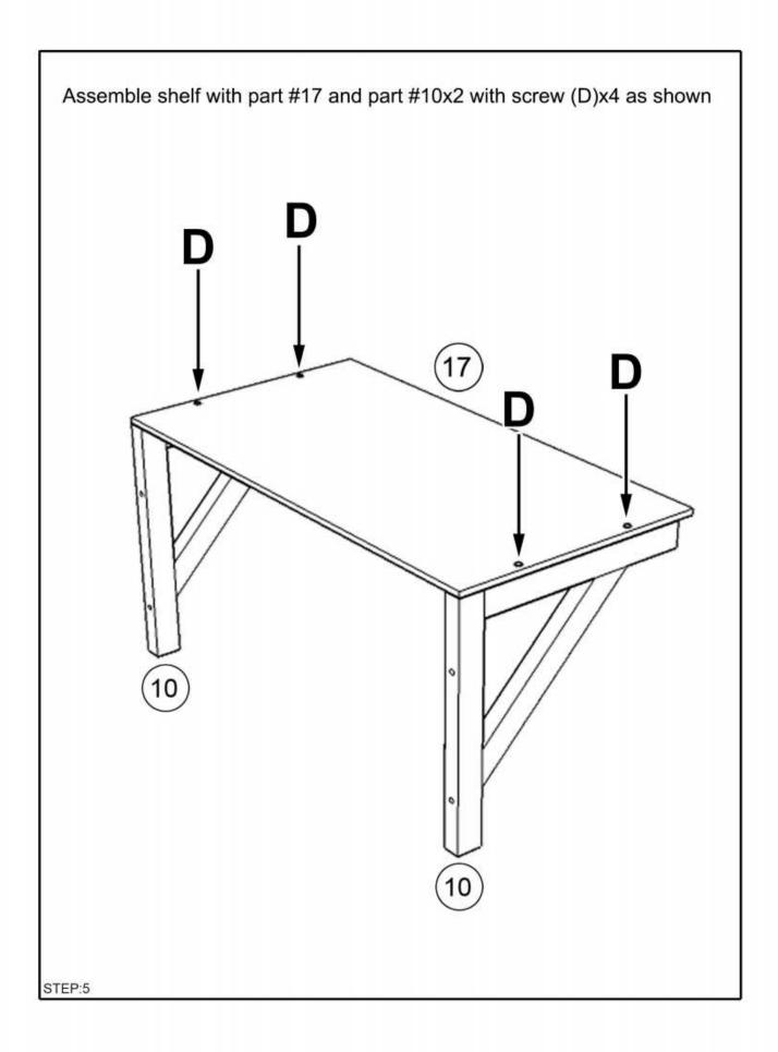
Requires two people to install the shelf at designated position, one person is inside the cage holding the shelf while the other person is outside locking the screws through the pre-drilled holes as shown X4
