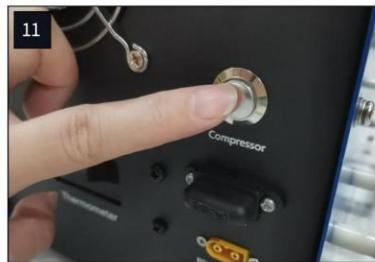
According to the size of the PCP airgun's air cylinder, its charge state and the target pressure, charging time will vary. Typically it will take approximately 25 minutes to charge an empty cylinder of 500cc capacity to 300BAR.
