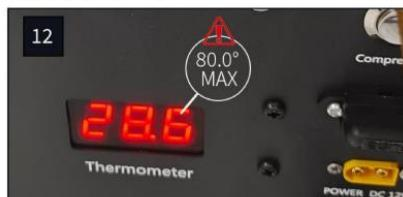
During the charging process, the temperature of the unit (in degrees Celsius) will be visible in the LCD display on the top of the main unit [fig 12]. This should be monitored throughout the charging process.
