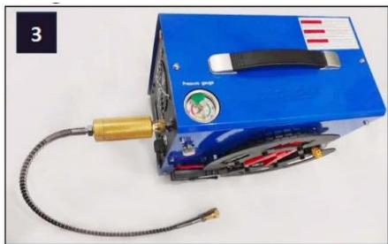
The hose assembly attaches to the PCP airgun at the other end via a Foster-fit. An additional adapter/ connector may be required [fig4] due to the many different types of filler-fittings used across PCP airgun makes (refer specific PCP manufacturer). Note: A thread-to-Foster adapter is included in the accessory pack [fig 5].
