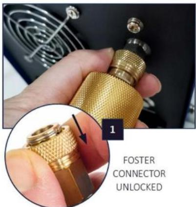
Note: Always double-check the connection is locked in place.
